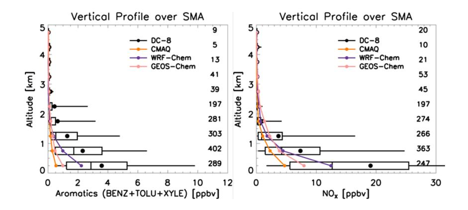
Comparison of NASA DC-8 observations with three independent models for aromatic VOCs (left) and NOx (right) over Seoul during KORUS-AQ.
