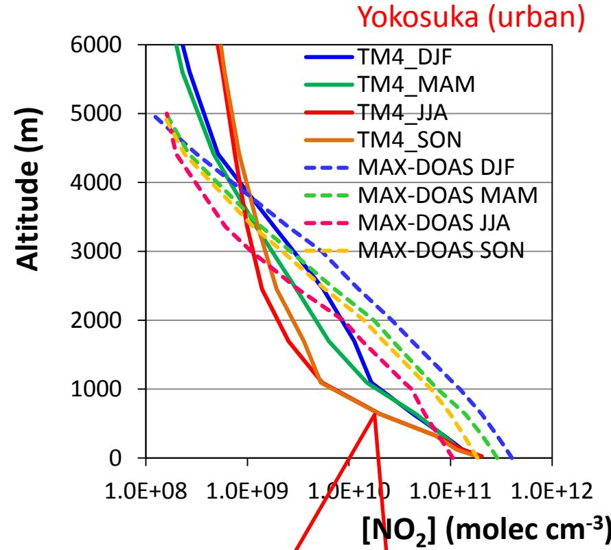
Rather steeper profile for TM4 than MAX-DOAS, despite coarse spatial resolution ( $2^\circ \times 3^\circ$ )
